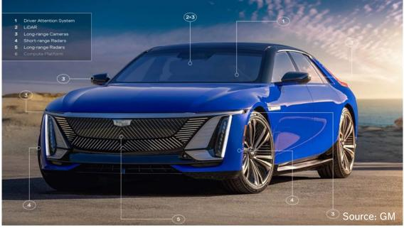
7 long-range cameras, 4 short-range and 3 long-range radars, 1 LiDAR, high-performance onboard compute for L2+ system... ... not being used on average 23h per day.
