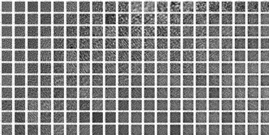
Figure 40 Real Ronchigrams with different defocus and aberrations. Each row represents a so-called focus stack, where focus was changed from under, in, to over focus. The top row has zero A1 aberrations, the bottom row the worst. Note that these are estimations done with a separate tool. The real microscope has no fixed state, all corrections are relative. Hence there is no real way to state that a lens is causing a certain known aberration.
