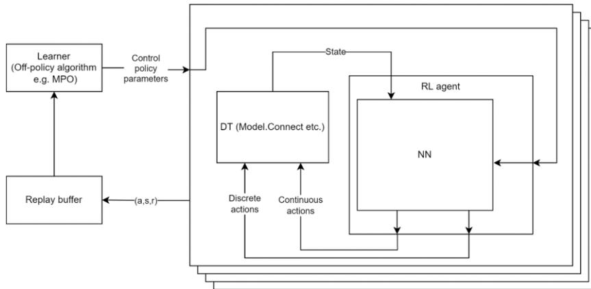
Figure 19 Architecture for the hybrid RL approach (actor-critic) in the UUV use case, inspired by [A2] and [A5]. Boxes denote components, arrows depict data flow. The layers on the right represent a set of distributed actor instances.
