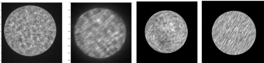
Figure 29 Domain mismatch example. The two left images are real Ronchigrams, the others are synthetic.
