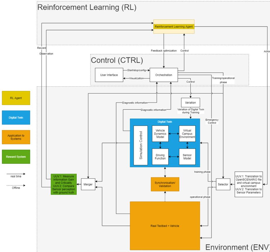
Figure 17 Architecture for the UUV use case (following the ASIMOV reference architecture). Boxes denote components, arrows denote data flow. Details of the artefacts most relevant to RL are provided in the text below.
