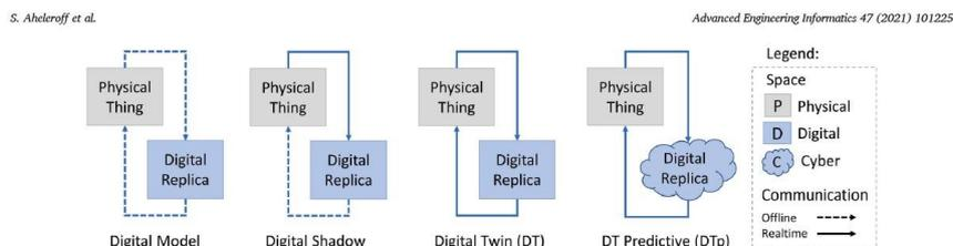
Figure 9 Illustration of the differences between a digital model, a digital shadow and a digital twin. Reproduced from [50].
