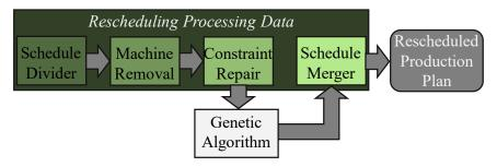
Figure 7 - Flowchart of ISEP's production plan rescheduling process for machine breakdown events.
