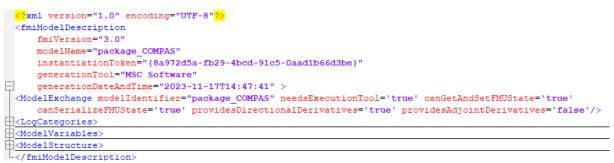
Figure 6: Sample excerpt of top level line of the XML file defining the FMU
