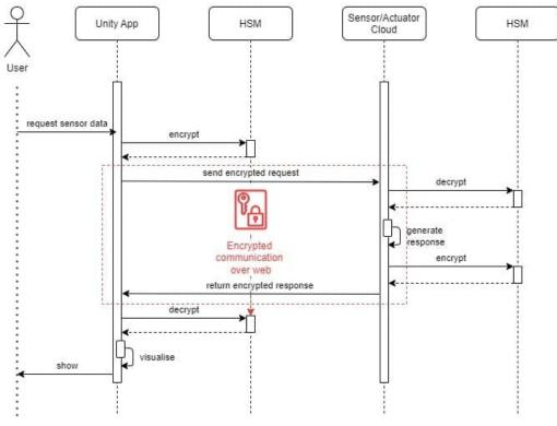
Figure 2. Encrypted data exchange between Client applications and Cloud
