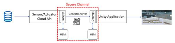
Figure 4. Encrypted data exchange between Client applications and Cloud.
