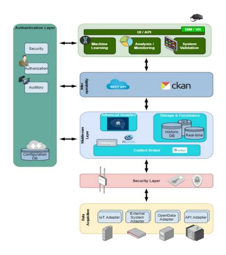
Figure 11. An example layered architecture for the management of smart buildings.
