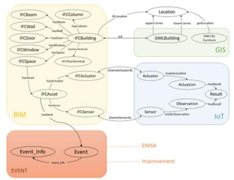
Figure 8. GIS-BIM-IoT-Event integrated super ontology.
