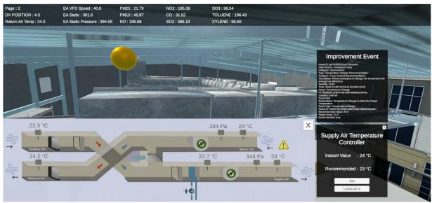
Figure 9. Event notification in the Unity-based Digital Twin application.
