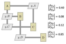
Figure 10: Example problem consisting of four disciplines with the corresponding sensitivity information [21].
