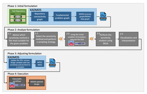
Figure 8: KADMOS MDAO workflow formulation process including global sensitivity analysis to identify noninfluential design variables [21].
