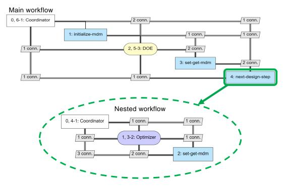
Figure 16: VISTOMS visualization of generated CMDOWS file for a nested multi-architecture optimization workflow calling GKN Fokker's 'MDM' KBE tool.
