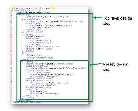
Figure 15: Example of Design Study Configuration file with nested design step
