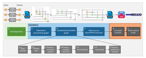
Figure 13: Overview of the workflow for implementing sensitivity analysis within the sequencing and decomposition algorithms.
