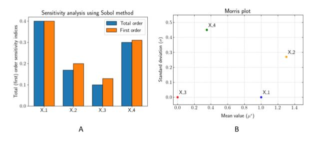
Figure 9: Example of bar plot showing total and first order sensitivity indices of input variables (A) and Morris plot of mean value versus standard deviation of input variables (B) [21].
