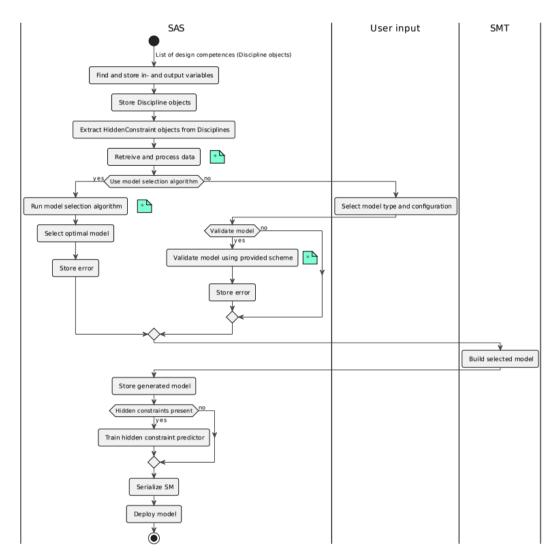
Figure 5: Activity diagram of the normal SM building procedure as implemented in SAS [16].
