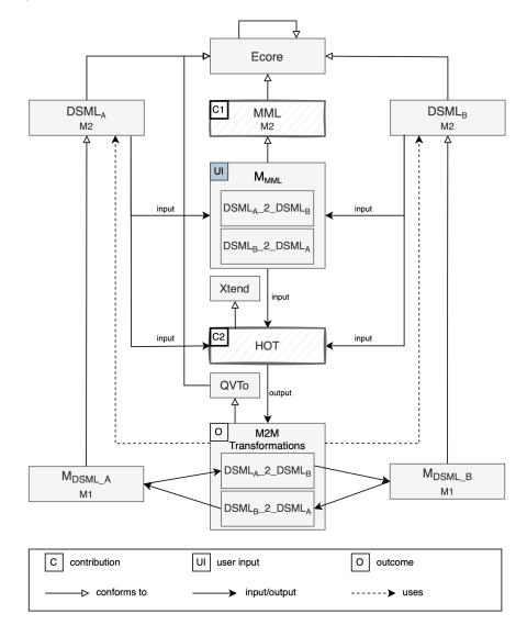
Figure 14 - Architecture for HOTs and bidirectional synchronisation
