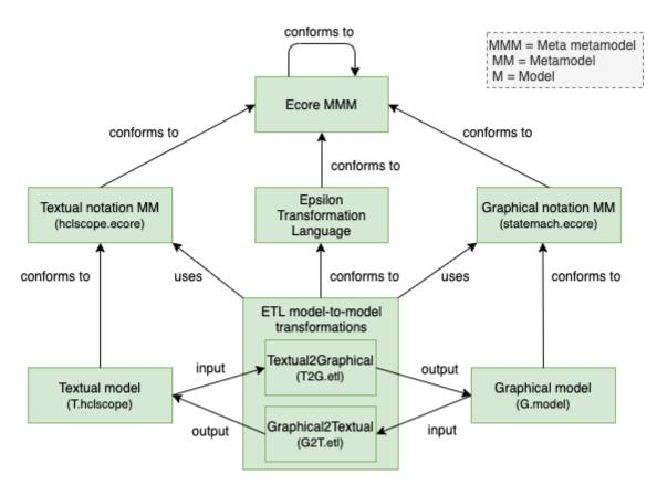
Figure 10: High-level architecture for the synchronisation between the graphical and textual notations for UML-RT state machines.
