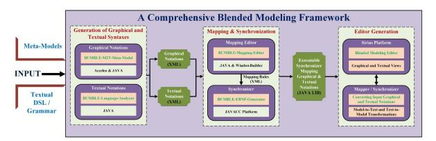
Figure 1 - The high-level architecture of proposed framework
