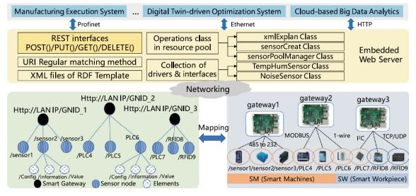
Figure 4. REST-based IIoT system
