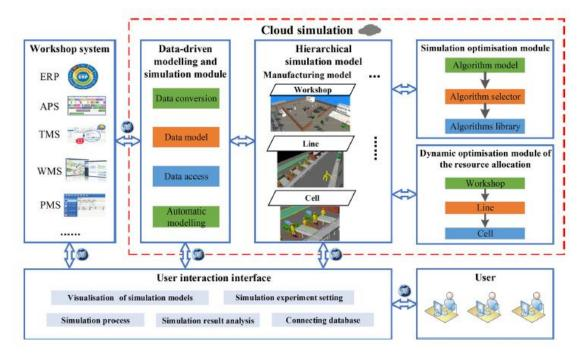
Figure 2. Data-driven cloud simulation architecture for AFPLs in smart factories.
