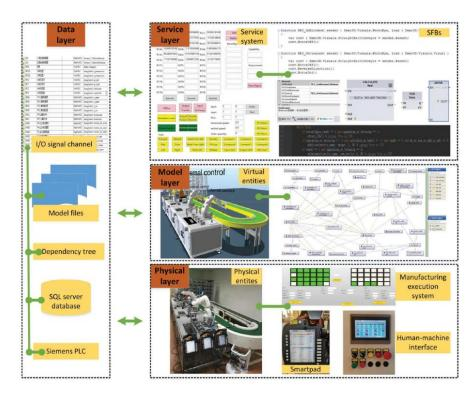
Figure 6. The structure of the prototype system.
