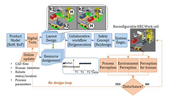
Figure 1. Paradigm on the design workflow of HRC applications.
