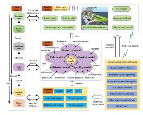
Figure 5. Five-dimensional fusion model-driven framework of RDTMS.
