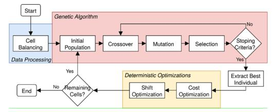
Figure 13. Flowchart of the ISEP production line scheduling system for total cost and machine longevity optimization.
