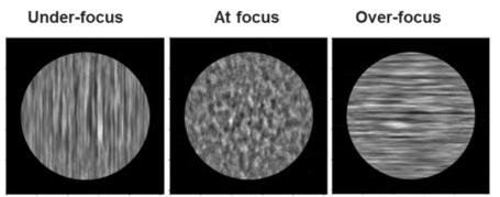
Figure 8 Response of Ronchigram image to 1st order aberrations, defocus and 2-fold Astigmatism: In presence of 2-fold astigmatism, Ronchigram pattern rotates by 90 degrees while changing focus settings.
