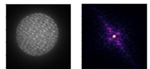
Figure 9 A Ronchigram image and its transformed form for two cases with different aberrations. Left: Only defocus is present, right: Both defocus and 2-fold astigmatism are present.
