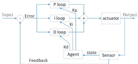
Figure 4 structure of RL-tuned PID controller.
