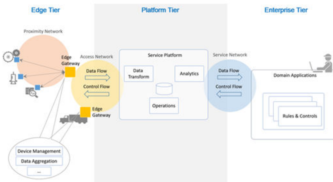
Figure 1. Three-Tier IIoT System Architecture
