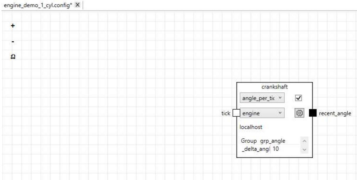
**Figure 16: Crankshaft emulation by angle calculation**
