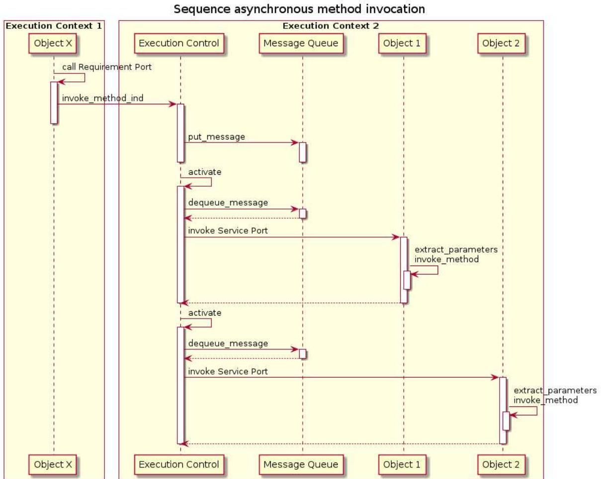
**Figure 4: Sequence of asynchronous method invocation**
