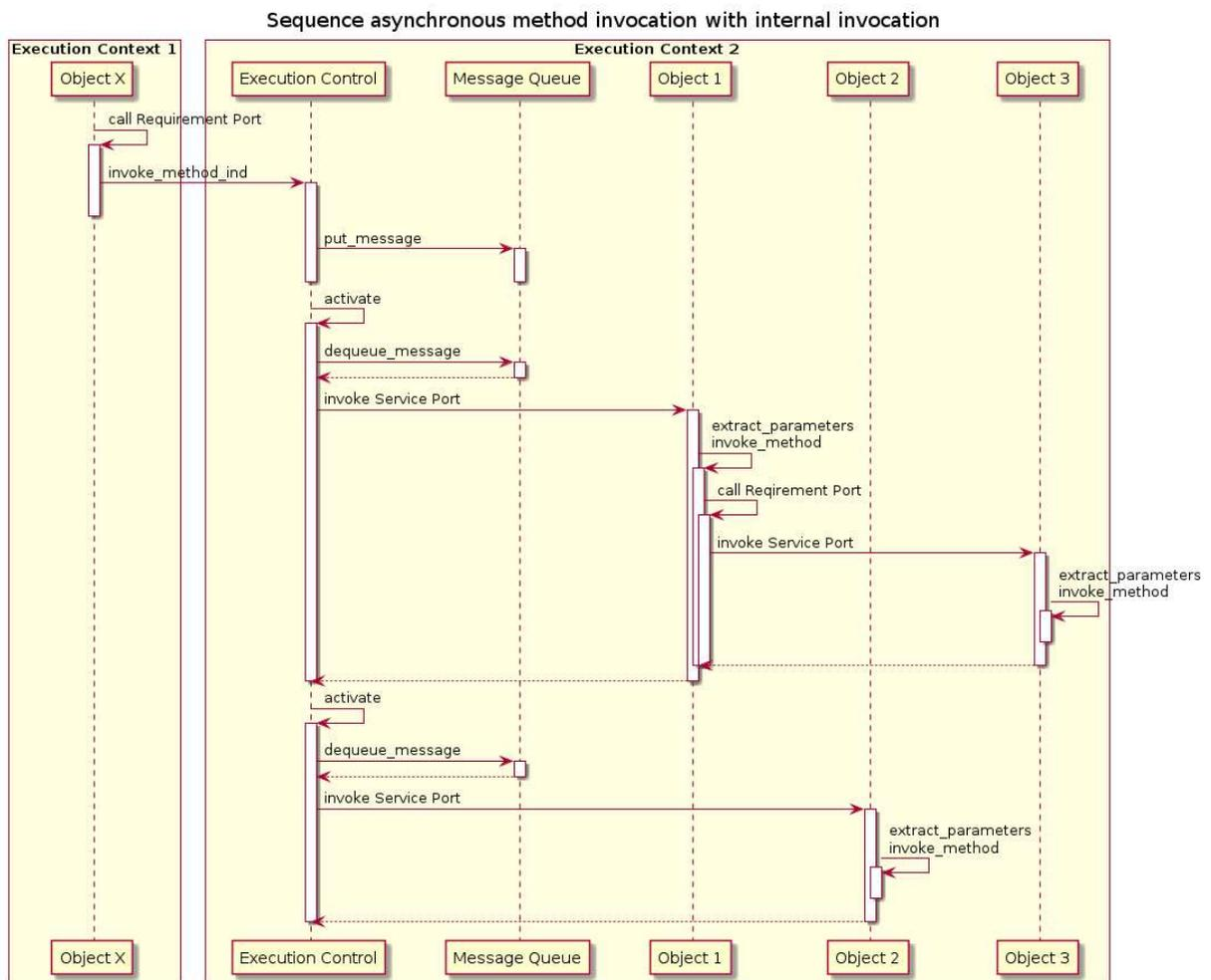
Figure 6: Sequence of asynchronous method invocation with internal invocation
