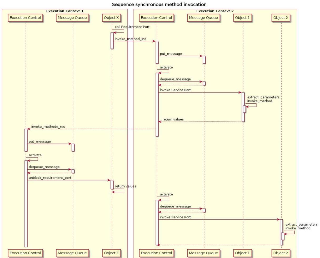
**Figure 7: Sequence of synchronous method invocation**
