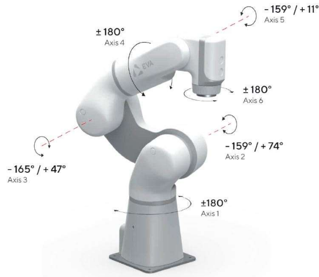
Figure 11. EVA 6 axes movements.
