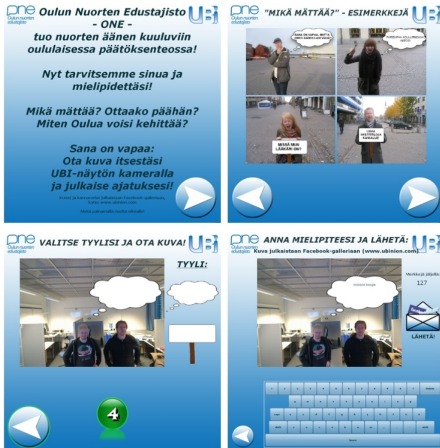
Figure 3. The four phases of the photography service. From top-left: instructions and description; example photos with captions; live webcam stream and camera button with countdown for taking snapshots; virtual keyboard for typing with a button for uploading the result to an online gallery.
