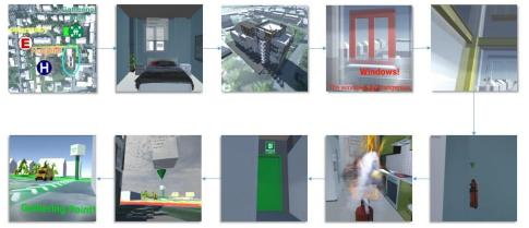
Figure 4: VR-based Earthquake Training including Fire Intervention
