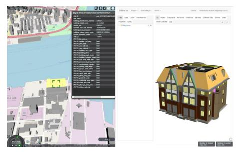
Figure 8: Screenshot on New York City's (City of New York, 2017) GIS model from 3DCityDB-Web-Client connected to the Schependomlaan BIM model (openBIMstandards, 2015) on BIMServer
