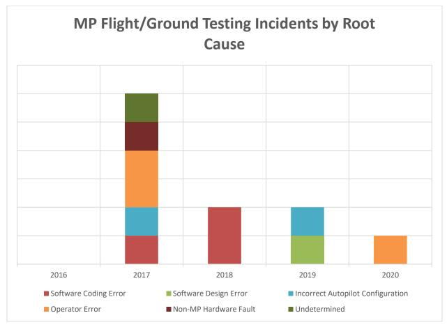
Figure 6 - MicroPilot Flight and Ground Testing Incidents by Root Cause
