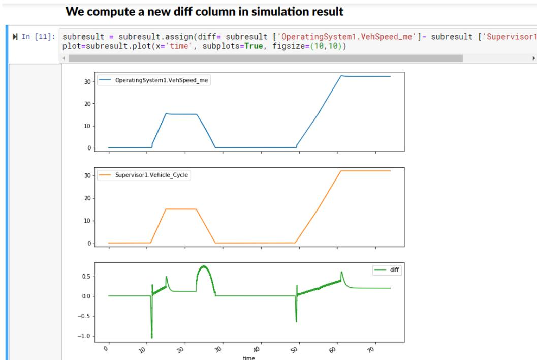
Figure 9 Creation of a new diff column in simulation results
