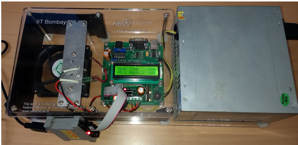
Figure 1: Single board heater system running a real-time control algorithm using firmware based on MDD code [Thi+17]).
