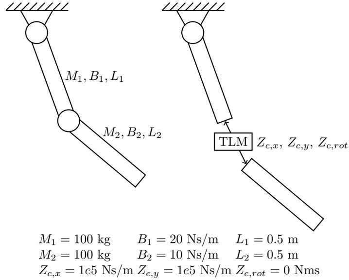
Fig. 5: A double pendulum is modelled as two arms connected by a TLM element. Impedance in the rotational dimension is set zero to allow free rotation.
