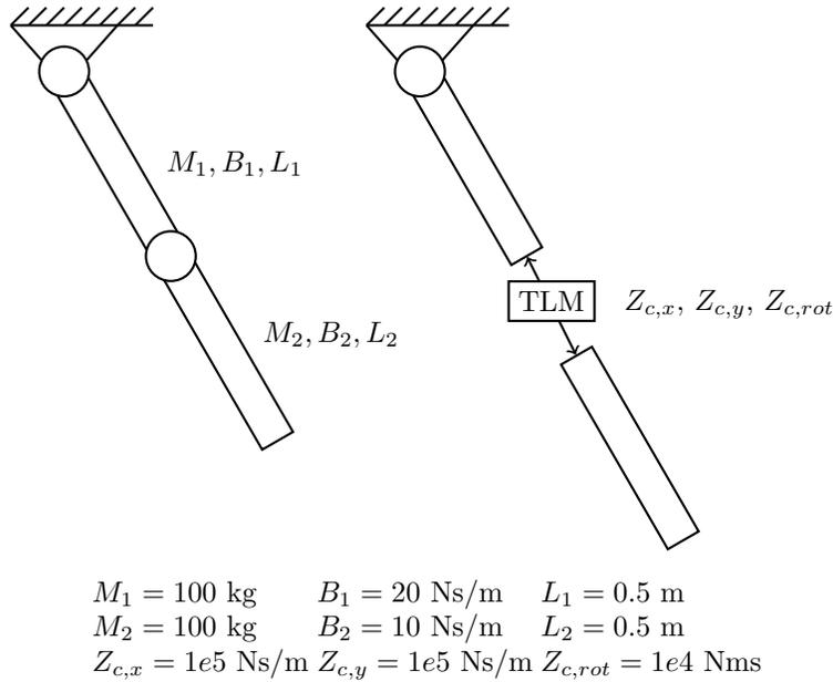
Fig. 7: A single pendulum is modelled as two arms connected by a stiff TLM element. Impedance is non-zero in all three dimensions.
