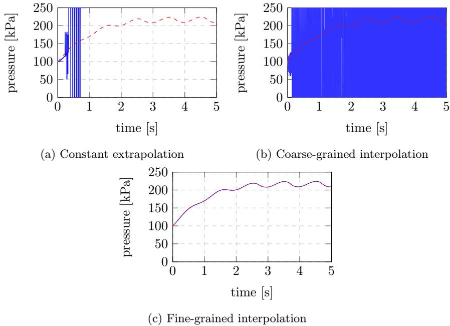
Fig. 10: Pressure in the TLM connection of the thermodynamic model. Dashed line is the Modelica simulation reference solution.
