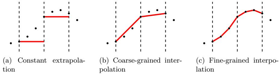
Fig. 2: Three variable estimation methods are used to stabilize the connections.
