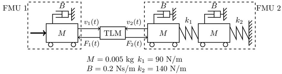
Fig. 3: A test model consisting of a three-mass system is divided into two FMUs.
