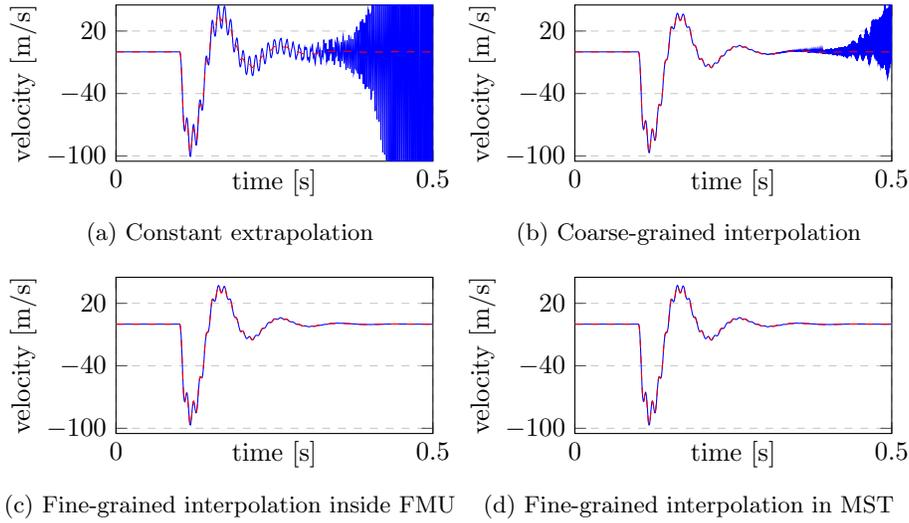
Fig. 4: Velocity against time at the left side of the TLM connection. Red dashed line is the exact reference solution.
