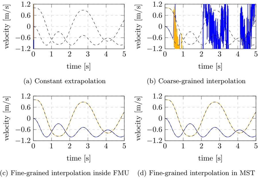
Fig. 8: Vertical and horizontal positions of the lower end of the single pendulum model. Dashed lines are the exact reference solutions.
