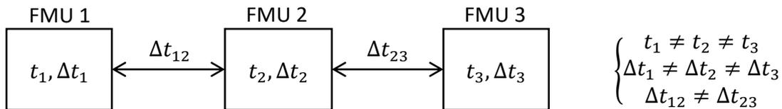
Figure 1: TLM connections enable independent solvers, time variables and step-size control.
