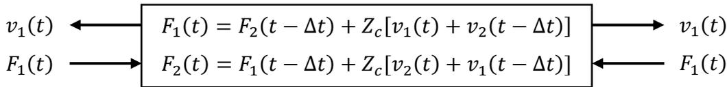
Figure 2: A TLM element with its equations.
