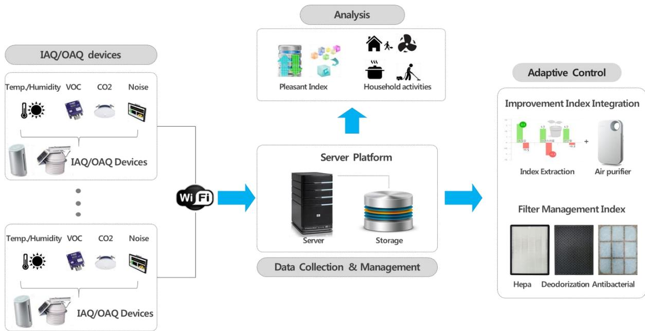
Figure 17. Main components consists of intelligent air quality management system.
