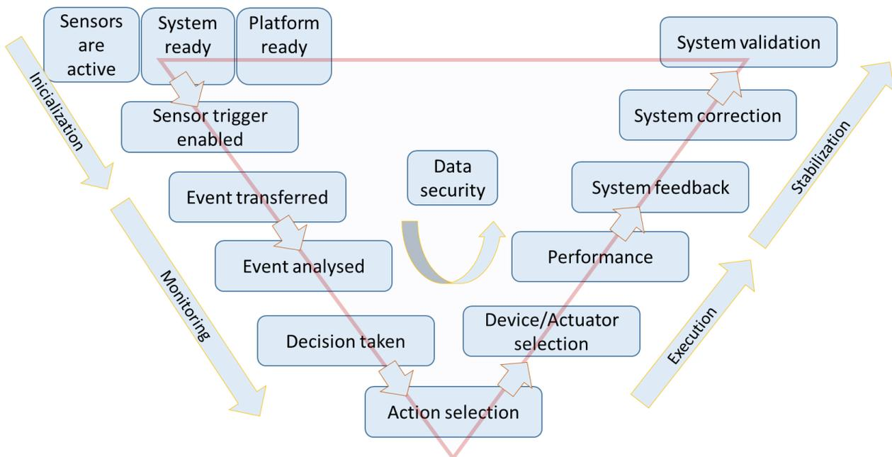
Figure 15. High-level function specification on the HVAC use case expressed by process V-diagram.
