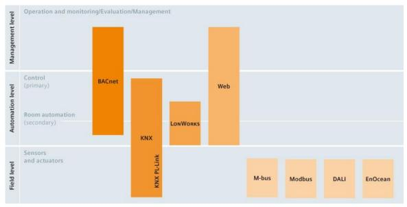
Figure 6: Communications protocols as used in the different levels of the automation pyramid [10]
