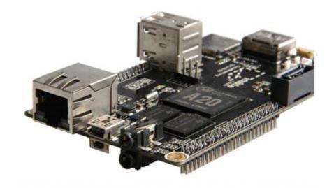
Figure 57: Singe-board computer Cubieboard2
