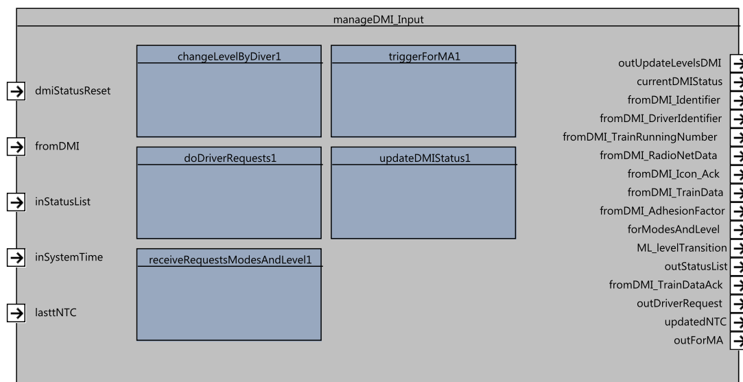
Figure 27. manageDMI_input SysML diagram.
