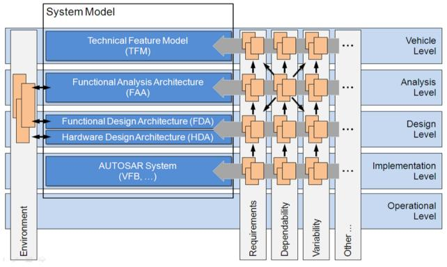
Figure 10: EAST-ADL levels and system model
