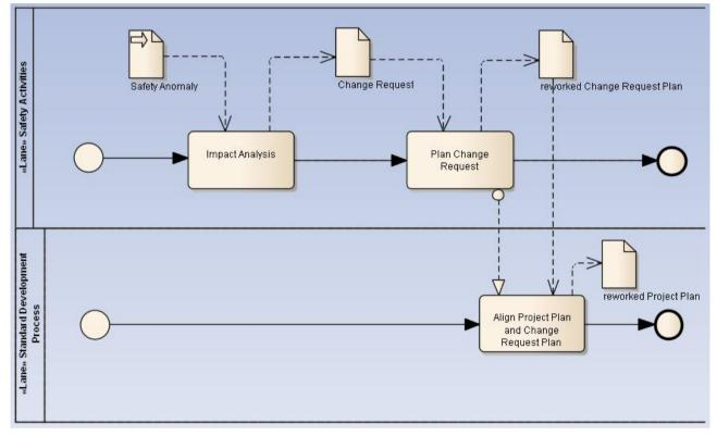
Figure 57: Basic Process Element for changes according "Safe"
