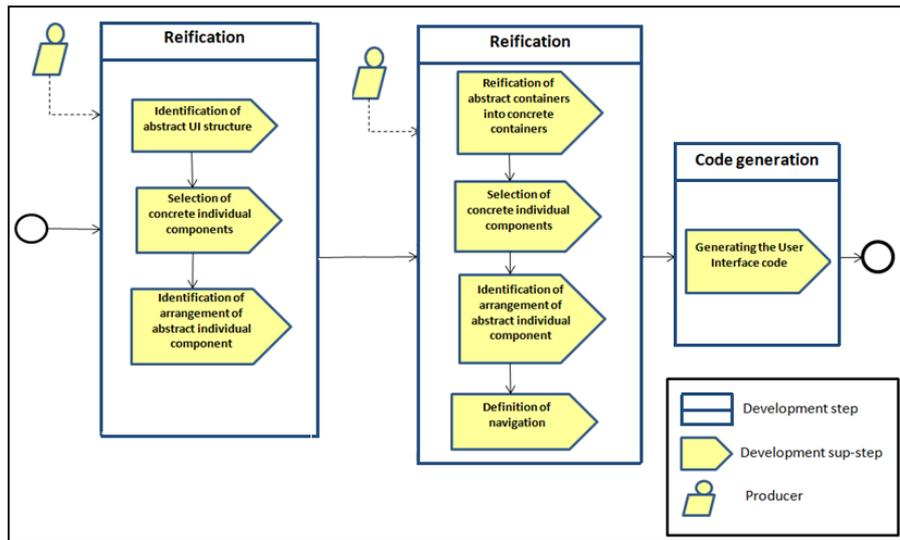
Figure 3. UsiXML Forward Engineering method expressed in SPEM4UsiXML
