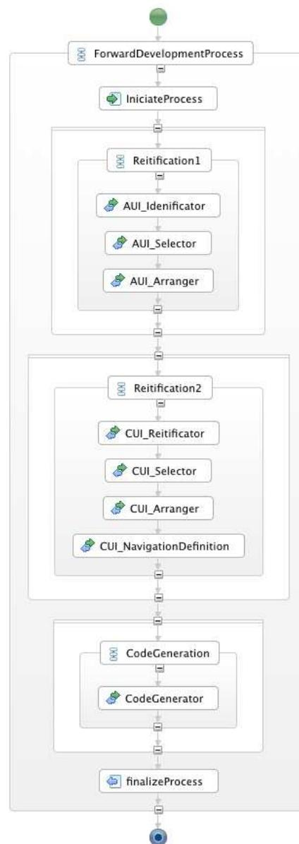
Figure A.7. *The BPEL Process of the UsiXML forward engineering method.*
