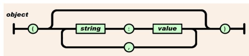
Figure: Object representation in JSON [1].
