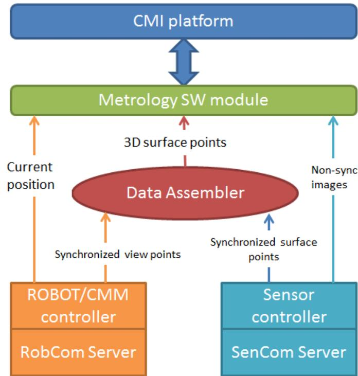
Figure 12: Communication architecture and information flow
