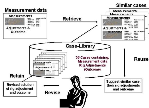
Figure 21: CBR applied to geometric production measurements (Volvo CE)
