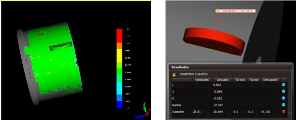
**Figure 15: Key analysis in the first metrology check**
