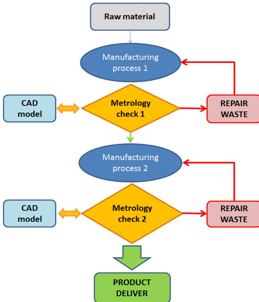
Figure 8: Industrial metrology demonstrator scheme
