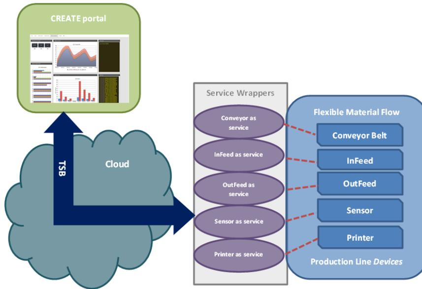
**Figure 3: Devices as web services in the demonstrator**
