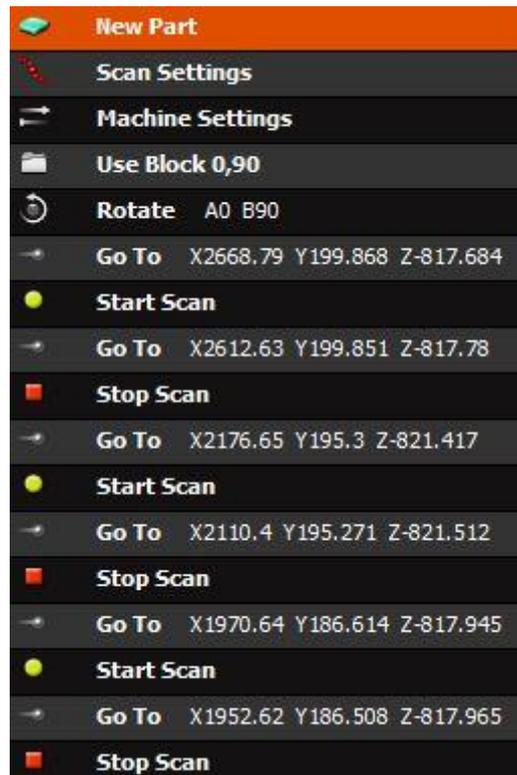
**Figure 13: Movements and trajectories for scanning**
