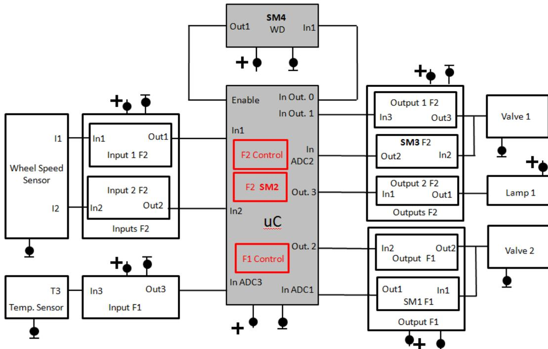
Figure 14: Technical Safety Concept for ISO26262-Part5 Figure E.1
