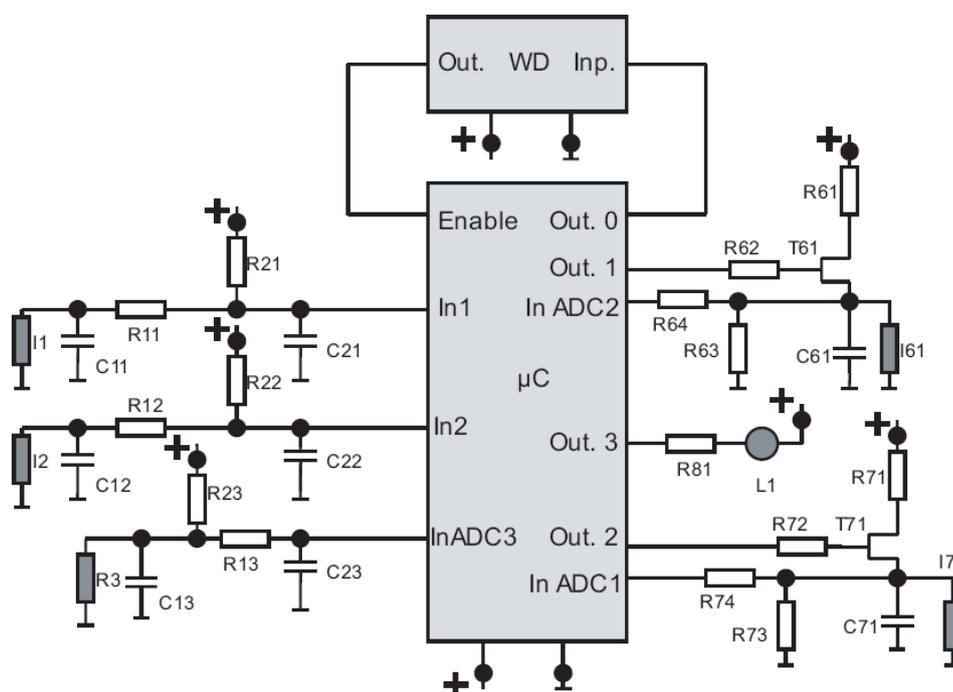
**Figure 13: Electronic Schematic diagram ISO26262-Part5 Figure E.1**
