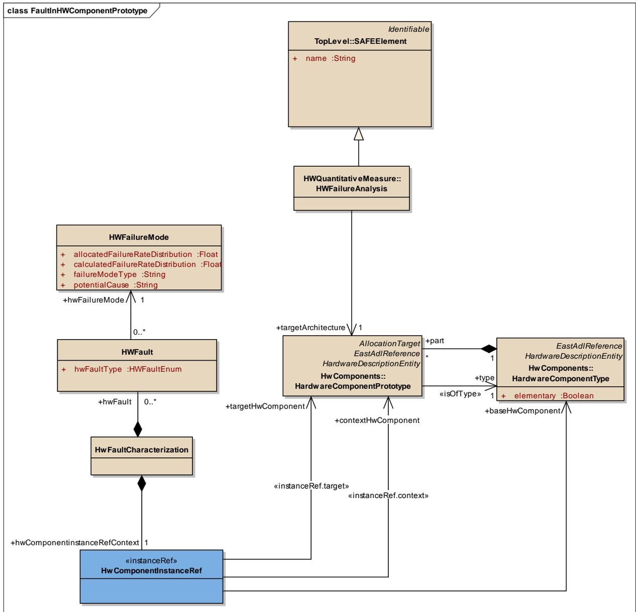
Figure 3: FaultInHWComponentPrototype - (Class diagram)
