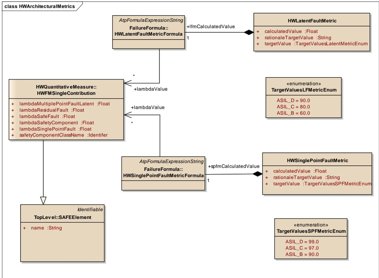
Figure 8: HWArchitecturalMetrics - (Class diagram)
