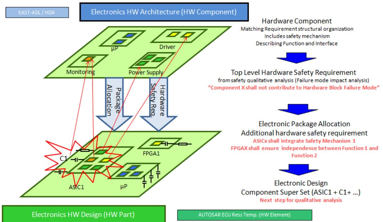
**Figure 4: Hardware allocation and quantitative analysis**
