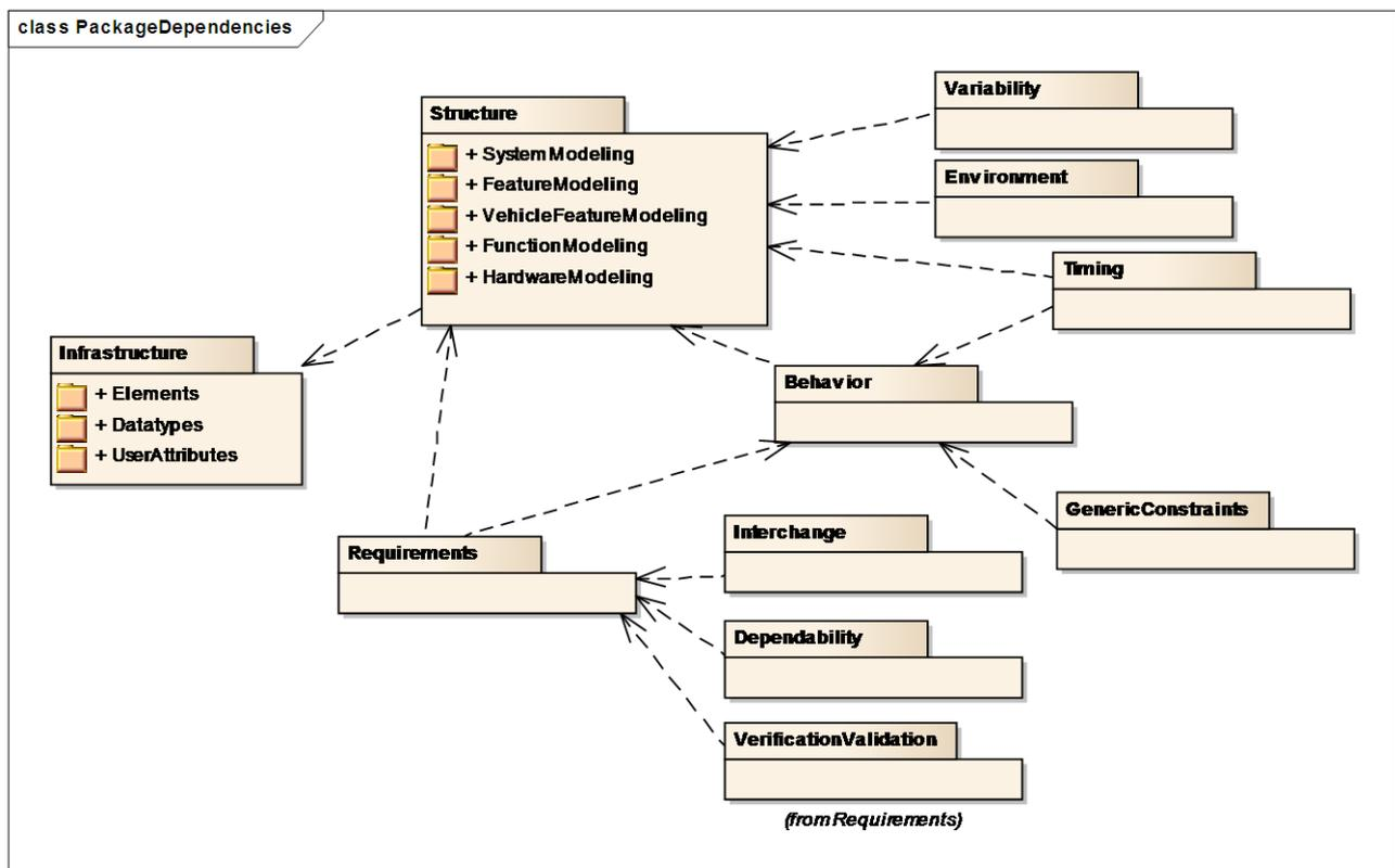
Figure 5: Class diagram for Package Dependencies
