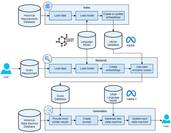
Figure 27: Pipepline of ReForm tool for automated model generation.
