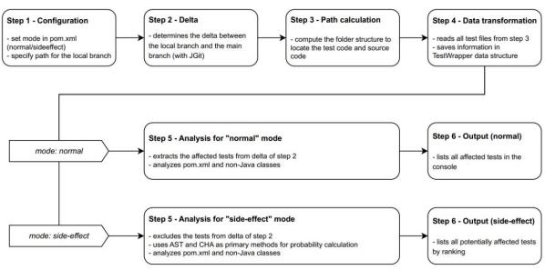
Figure 90: High-level workflow of CBTS
