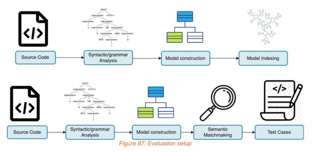
The evaluation of SONATA was conducted using a two-phase approach that tested both its core functionalities: model extraction and semantic matchmaking. The setup was designed around two key components, as illustrated in the diagrams:
