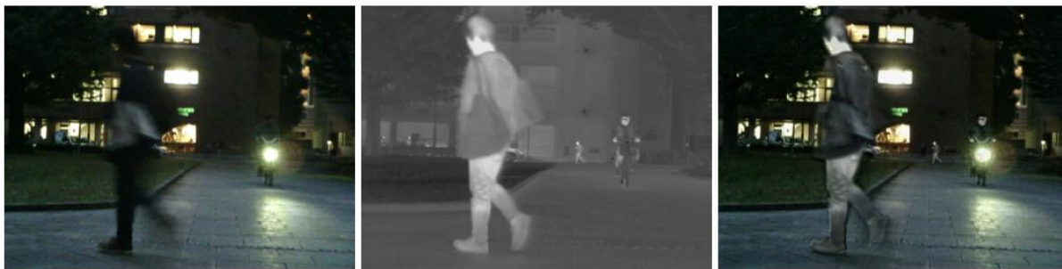
Figure 9. An example of visual and thermal imaging fusion in low light conditions, with (left) visual input, (centre) thermal input and (right) a resulting fused visual-thermal image
