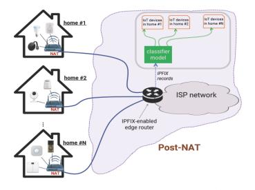
Fig 4 The Architecture of Pashamokhtari et al. Solution. Image Source: [Pashamokhtari-2021]
