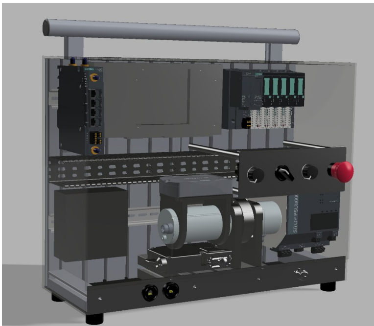
Figure 2: Electric motor with imbalance demonstrator
