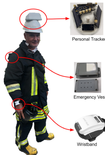
◀ Set of wearable orientation sensors consisting of three main devices: a wristband, a helmet and a gateway.
