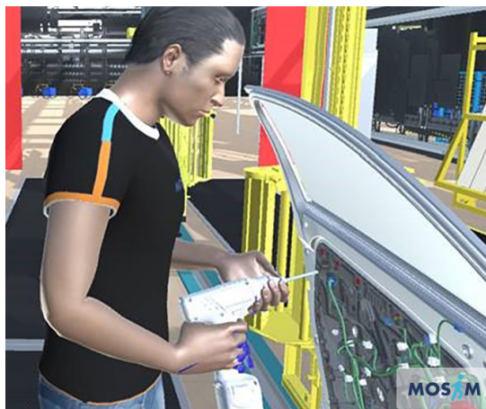
Example for the automotive industry: MOSIM enables the automatic simulation of manual assembly processes.
