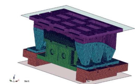
*Simulation of the solidification of a break disc pattern (MAGMA)*
