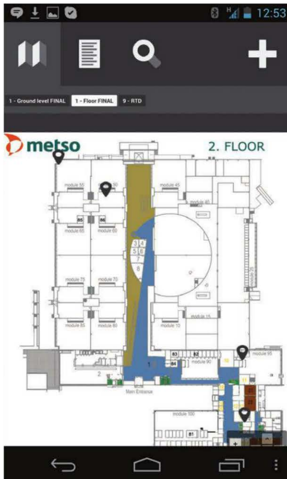
The smartphone handset guides a maintenance technician through a complicated plant layout to a point where a service action is required
