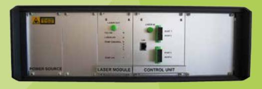
*Figure 2* Interrogation system with built-in broadband light source, spectrum analyser and four FBG sensor multiplexer
