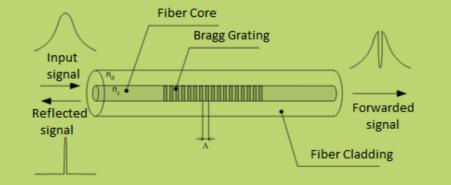
Figure 1 Fiber Bragg Grating function description
