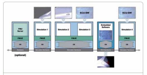
Basic idea of Functional Mock-up Interface for flexible and standardised simulator integration
