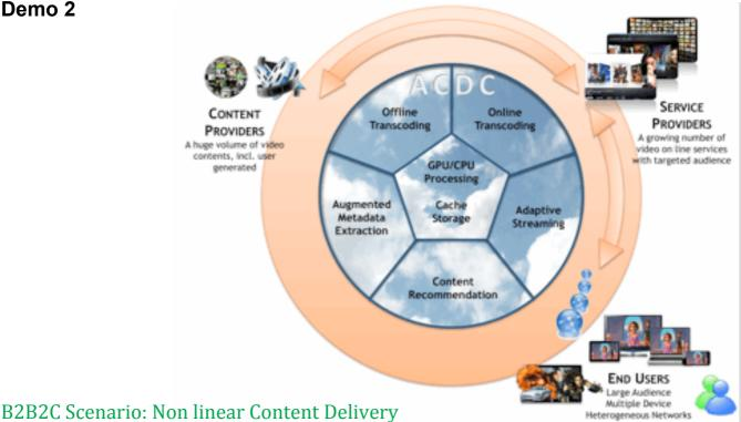
The present scenario illustrates the Adaptive Content Delivery Cluster concept, with the Proof-of-Concept of a complete eco-system relying on a shared cloud infrastructure powering new-gen Media and Semantic Services.
