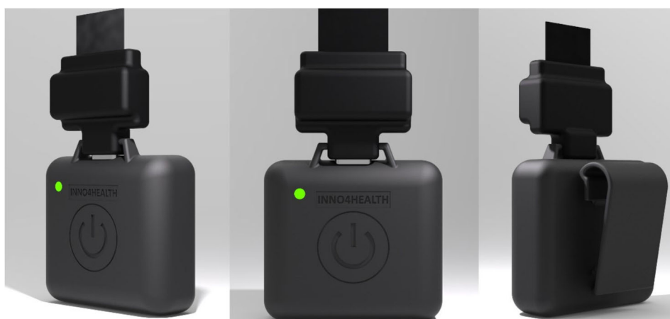
Figure 7 - Re-designed Insoles sensor inter-connection to electronics enclosure
