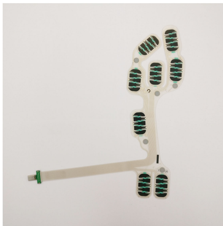
Figure 1 - RAW sensor after printed
