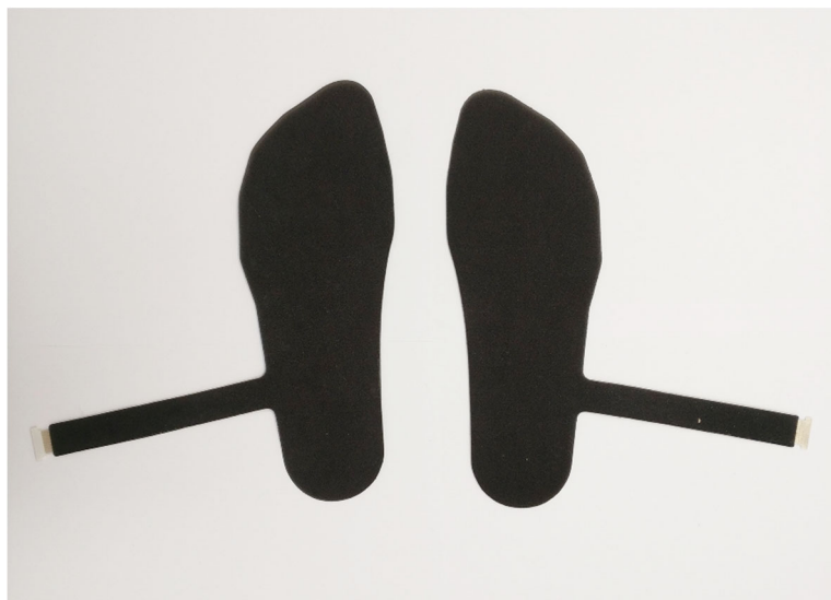
Figure 4 - RAW sensor laminated into two layers of Alcantara
