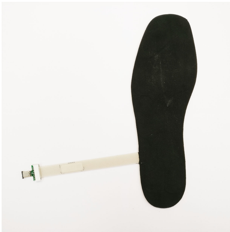
Figure 2 - RAW sensor laminated into two layers of natural leather
