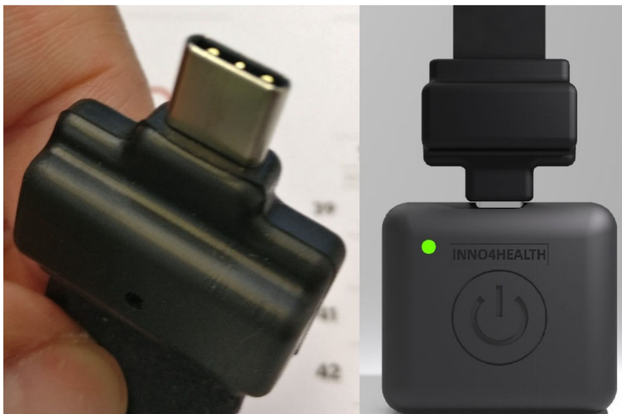
Figure 6 - Initial Insoles sensor inter-connection to electronics enclosure
