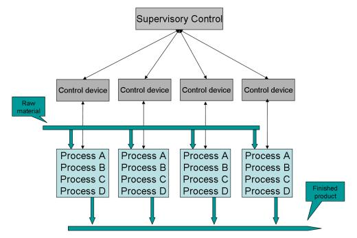
Figure 3 - Distributed automation system
