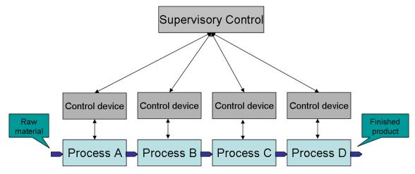
Figure 2 Multi layer centralized automation control
