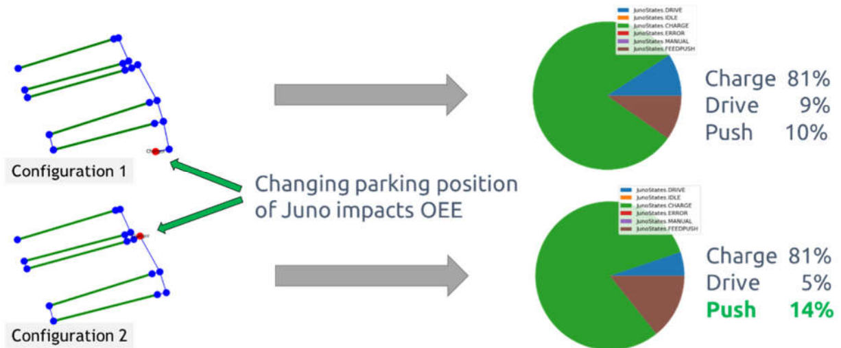
Figure 10: Example of different parking positions and how it influences the OEE parameters.
