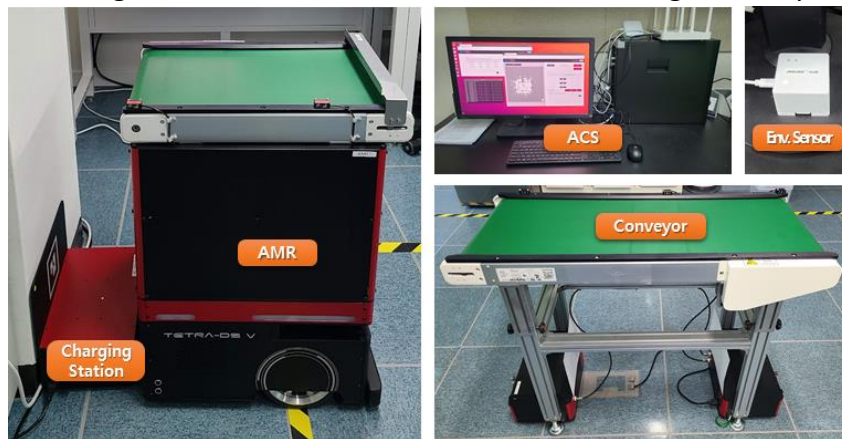
Figure 2. Hardware components of the indoor logistics testbed
