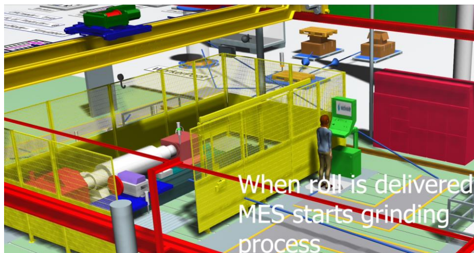
Figure 12 Roll is delivered by the crane. MES starts the grinding process.
