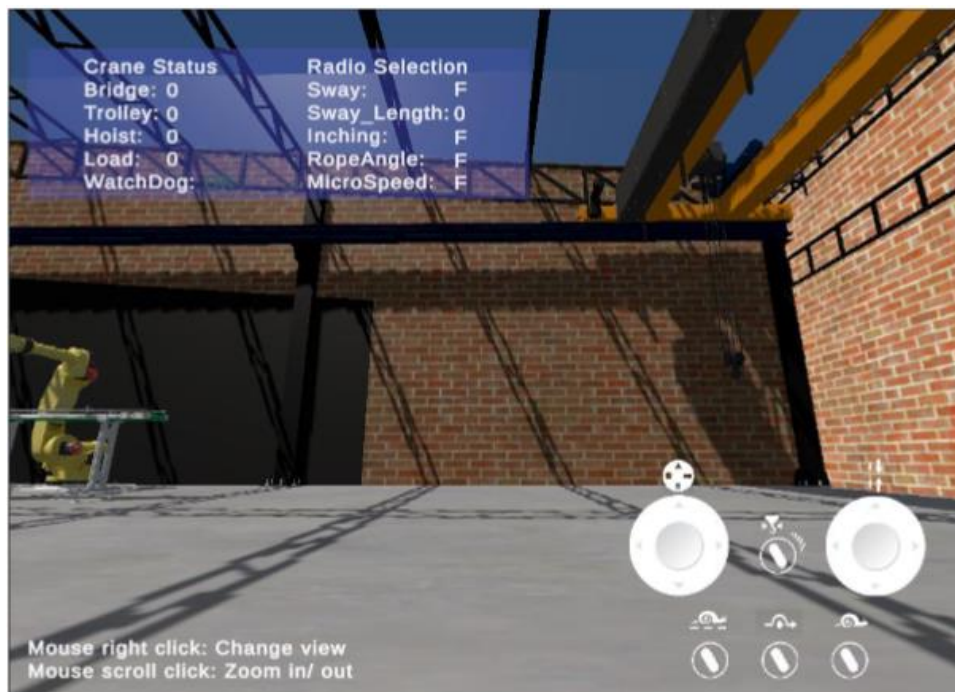
Figure 19 The screenshot of the remote-control prototyping app. The 2D remote controller is located in the lower and right corner.
