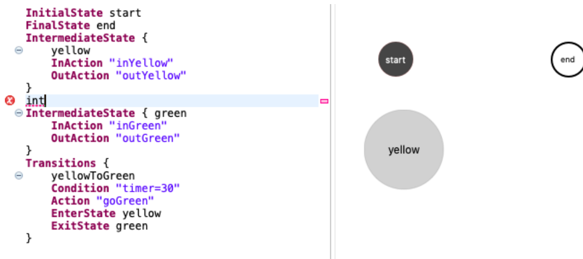
Figure 7: State of the editors after the syntax error with an automatic refresh strategy
