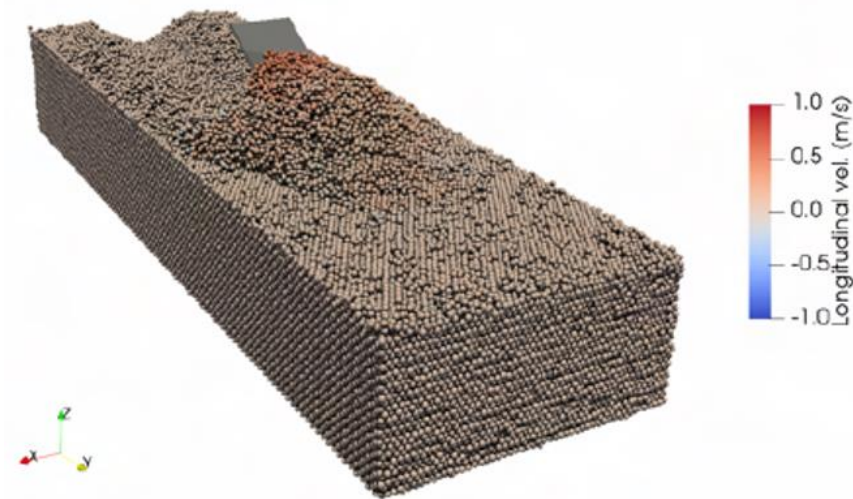
Figure 22: Example of one of the simulated tests in sand with 317780 bodies using a blade at 0,1 m depth.
