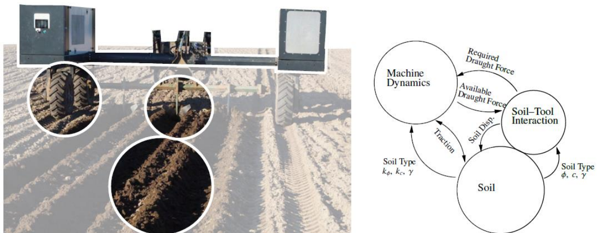
Figure 21: Graphic of the dynamics between the soil, machine and tool [27].
