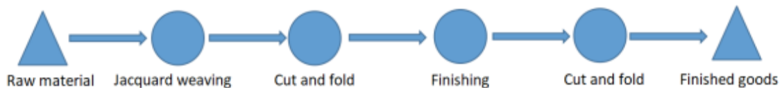
Figure 1. Jacquard production process
