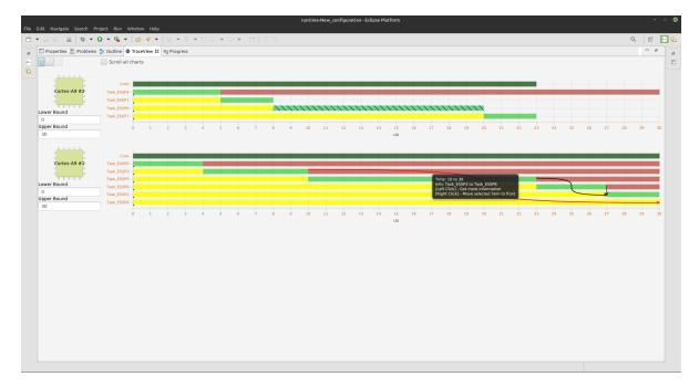
Figure 3.2: Gantt-Chart illustrating the execution of 10 tasks, including data propagation between the labels shared among those tasks
