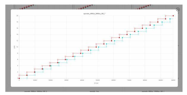
Figure 5.6: Detailed view of the trigger pattern generated by a relative periodic stimulus, which starts to draft for larger time intervals
