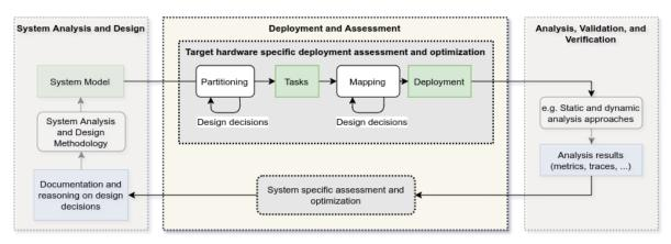
Figure 1.1: High-Level overview of a typical design flow within mobility systems development
