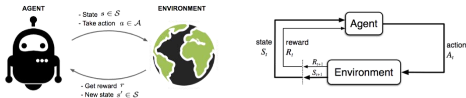
Figure 1 The basic elements of a reinforcement learning setup. Adapted from [99]
