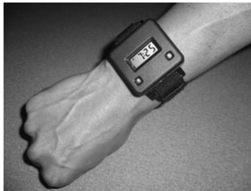
Fig. 7. Bite-counting device worn on the wrist in 'time' mode. [51]
