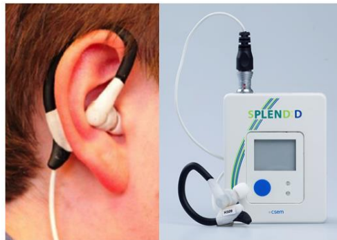
Fig. 6. First wearable version of the SPLENDID eating detection sensor (left: the eating detection sensor; rith: the eating detection sensor and datalogger). [42]
