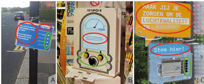
Fig. 2. The call-to-actions (marked in red) are designed to attract the attention of passers-by and can be combined with the interface itself (marked in green), such as in A) Postervote [62] and B) Viewpoint [55], or partially split-off into separate elements, as depicted for C) Citizen Dialog Kit [11].
